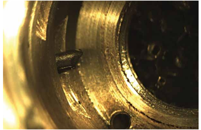
The coupling was not checked for this high speed handpiece; part of an O-ring has broken off, travelled down the drive air and damaged the turbine – expensive.
